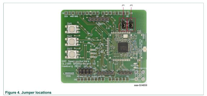
By default both board jumpers are set to the 1-2 position. Because the board only functions at 3.3 V, the jumpers must remain set to the 1-2 position. Do no move the jumpers to the 2-3 position.
