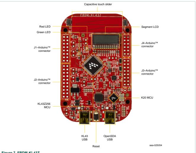
Figure 7 shows a top view of the FRDM-KL43Z and highlights its main components.
