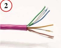
Untwist the pairs and Straighten the Wires
