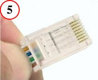
Insert Wires Along Plug Top, Maintaining Correct Alignment
