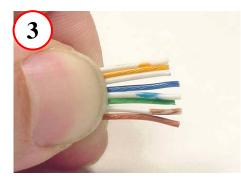
**Position Wires into Correct Configuration (568-B Shown)**
