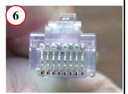
Inspect The Plug; Wires Should Be Visible from Plug Front
