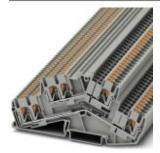
Double-level terminal block, Cross section: 0.14 mm<sup>2</sup> - 4 mm<sup>2</sup>, AWG: 26 - 12, Connection type: Push-in connection, Width: 5.2 mm, Color: gray, Mounting type: NS 35/7,5, NS 35/15
